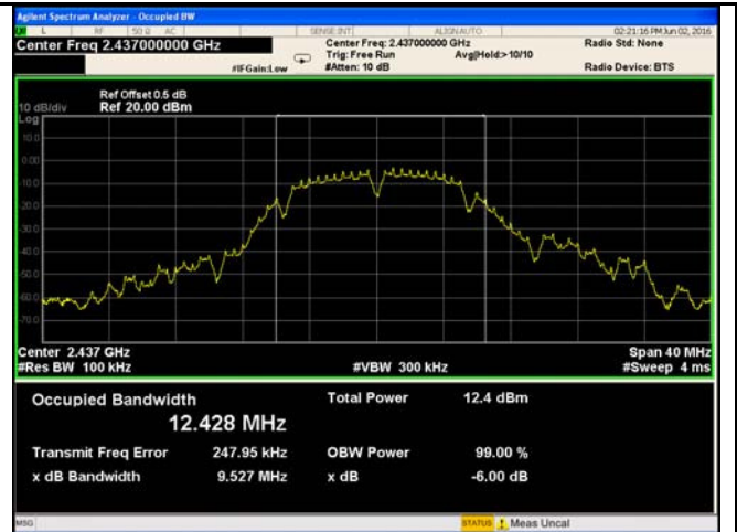
802.11b 6dB Bandwidth - Mid CH 2437
