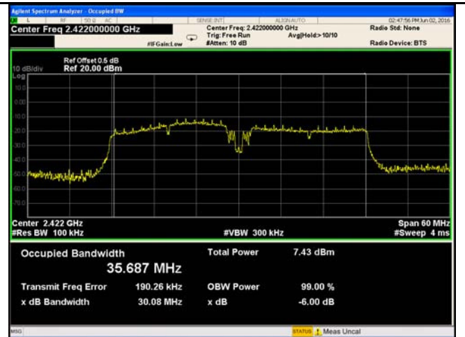
802.11n40 6dB Bandwidth - Low CH 2422
