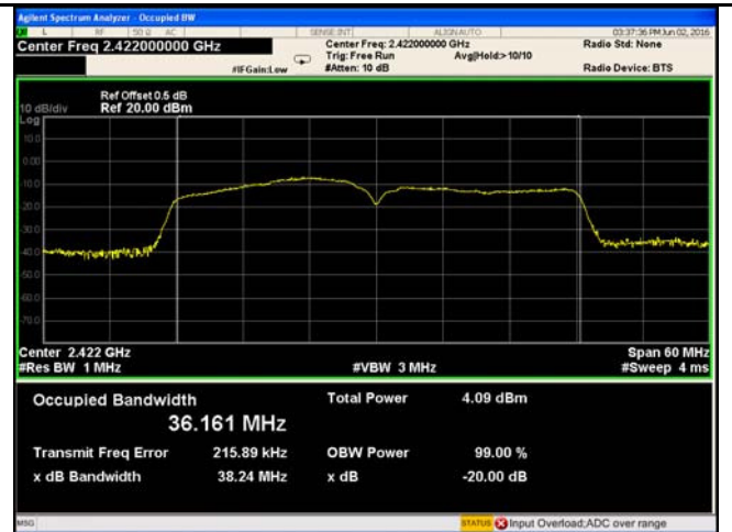
802.11n40 20dB Bandwidth - Low CH 2422
