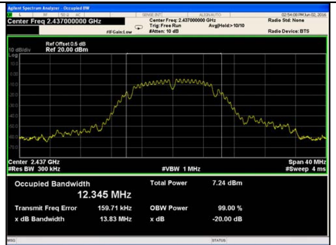
802.11b 20dB Bandwidth - Mid CH 2437
