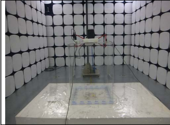
Radiated Spurious Emissions Test Setup Below 1GHz
