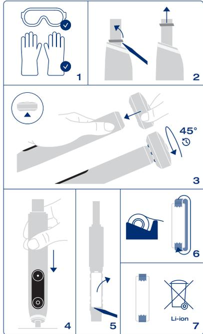
**Open the handle as shown, remove the battery and dispose of it according to local environmental regulations.**
