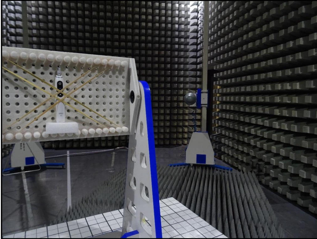
Photo 1 Radiated Test Setup XY plane
