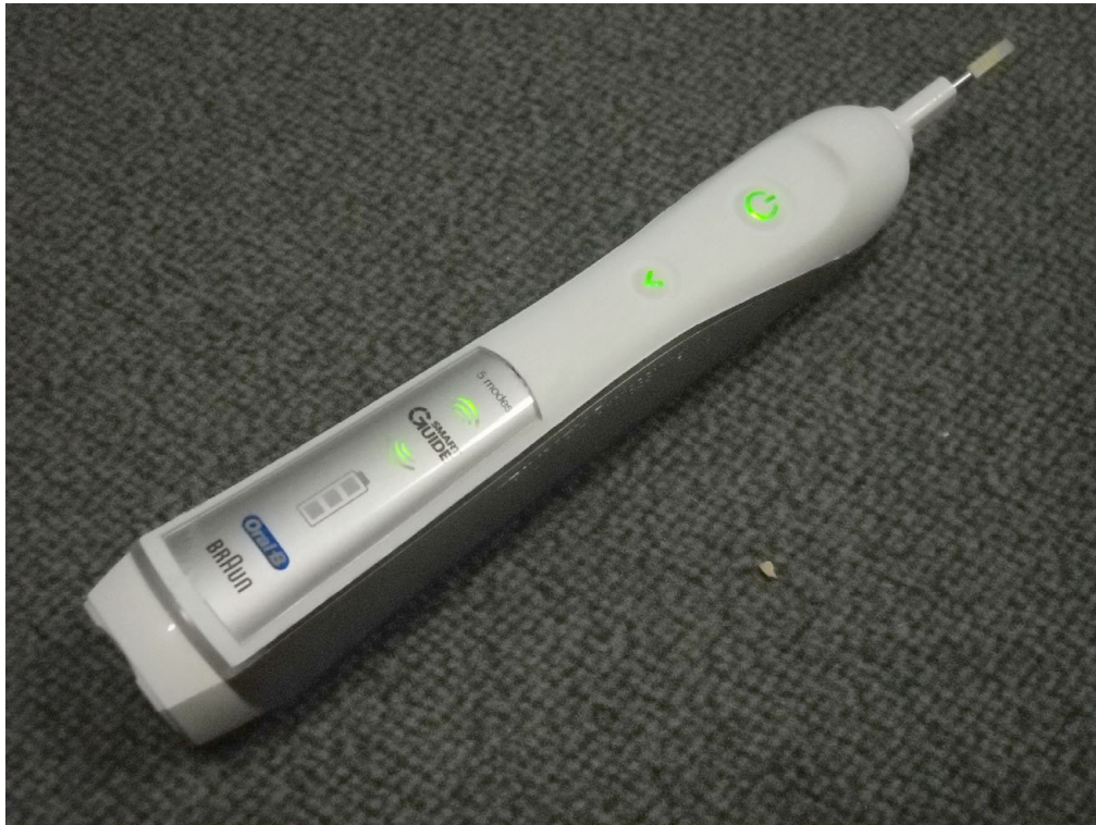
Figure 4 Tooth brush handle 3762 in brushing mode with RF transmitter on
