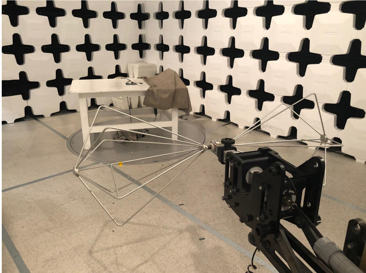
Figure 3. Radiated Emissions Test Configuration (30-200 MHz)
