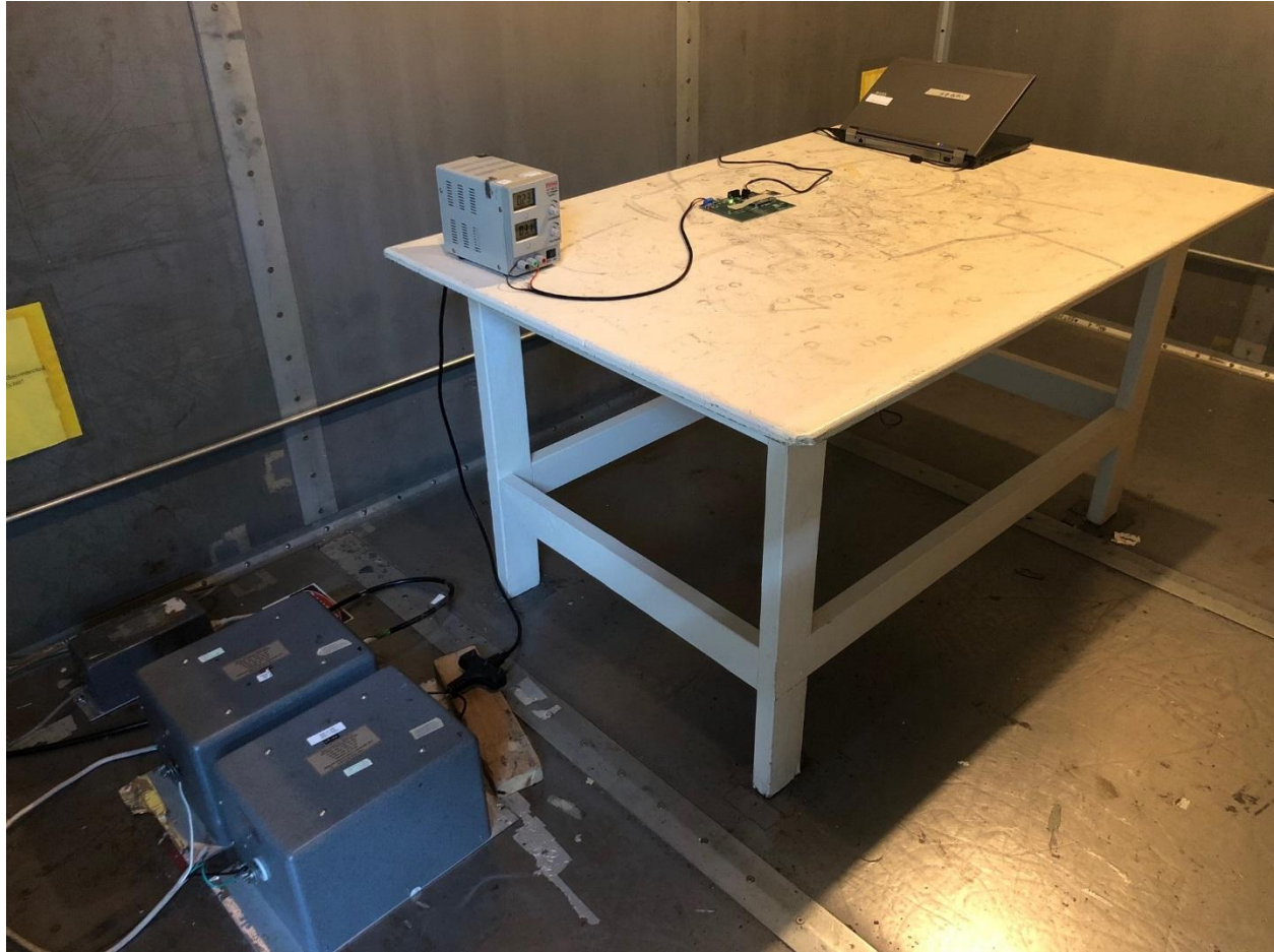
Figure 7. Power Line Conducted Emissions Test Configuration
