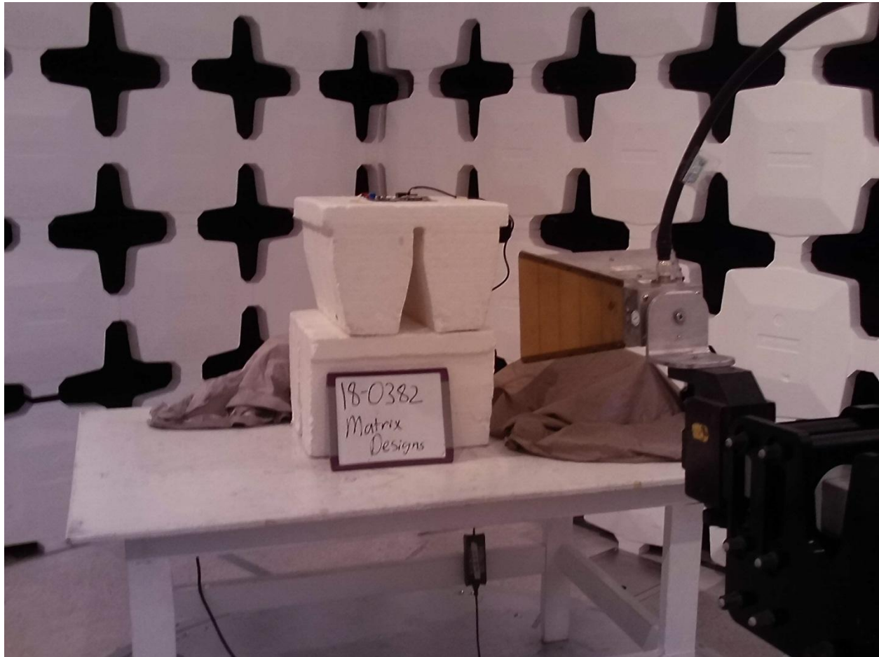
Figure 6. Radiated Emissions Test Configuration (Above 6 GHz)
