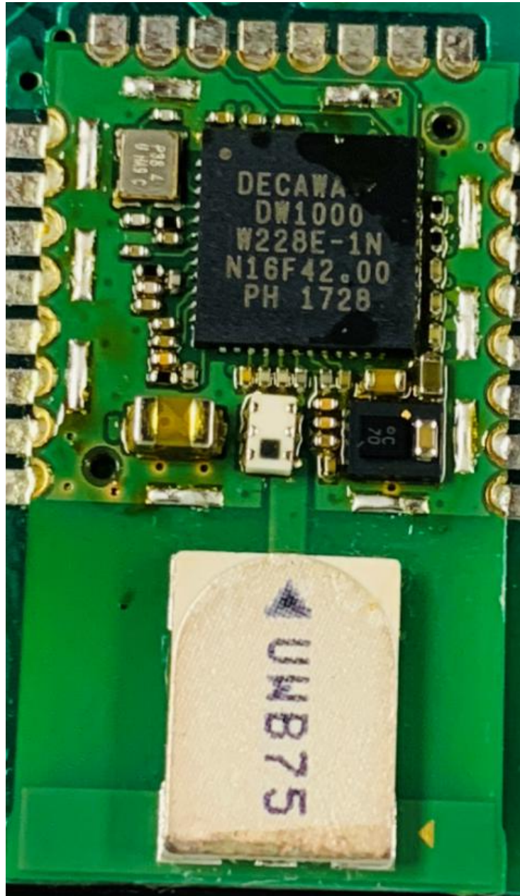
Figure 6. Close-up of Module without Shield
