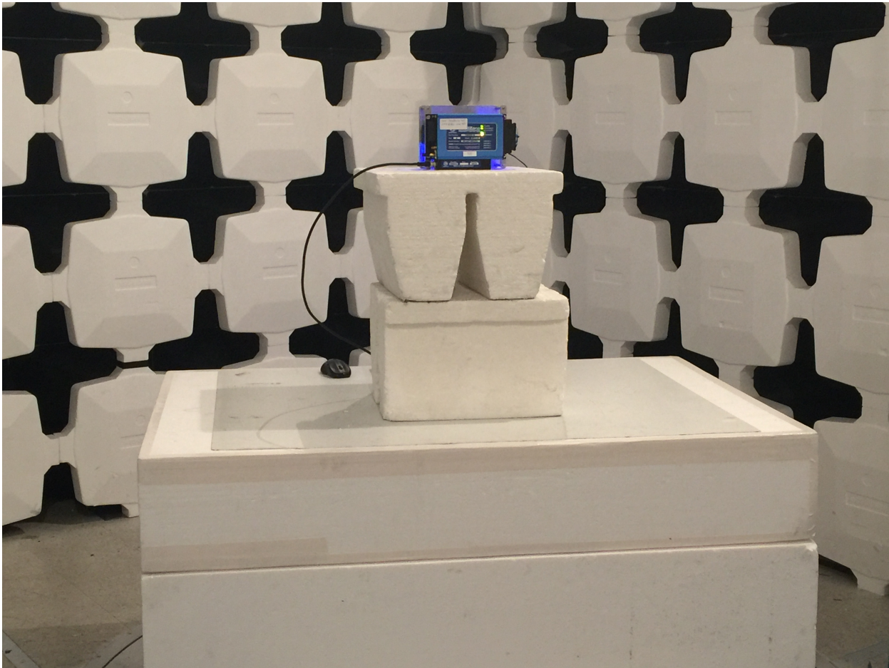
Figure 1. Radiated Emissions Test Setup, Close-up
