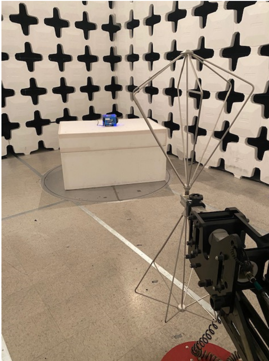
Figure 3. Radiated Emissions Test Setup, 30 MHz to 200 MHz
