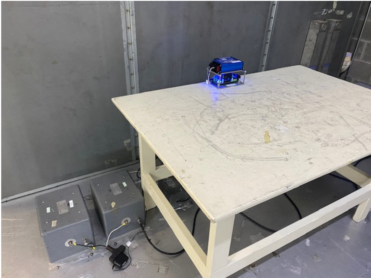
Figure 6. Conducted Emissions Test Setup
