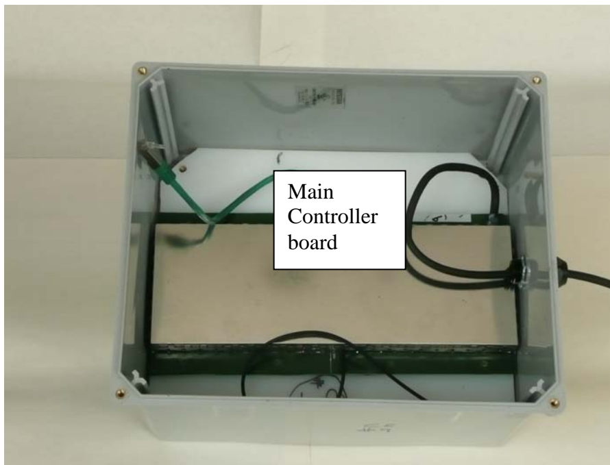
Contents removed, showing Main Controller board.
