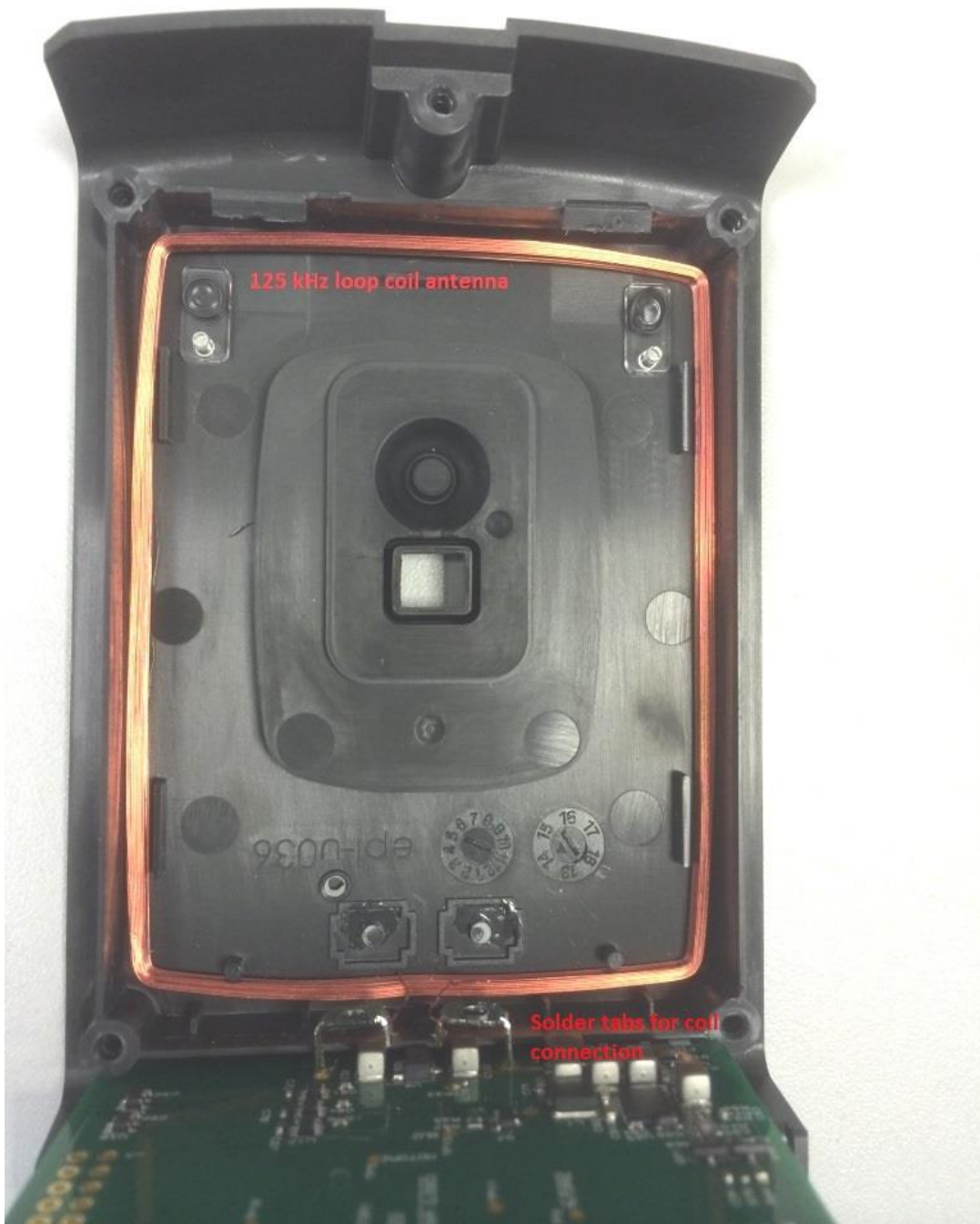
Housing lid with PCB pulled up to reveal 125 kHz loop coil antenna.
