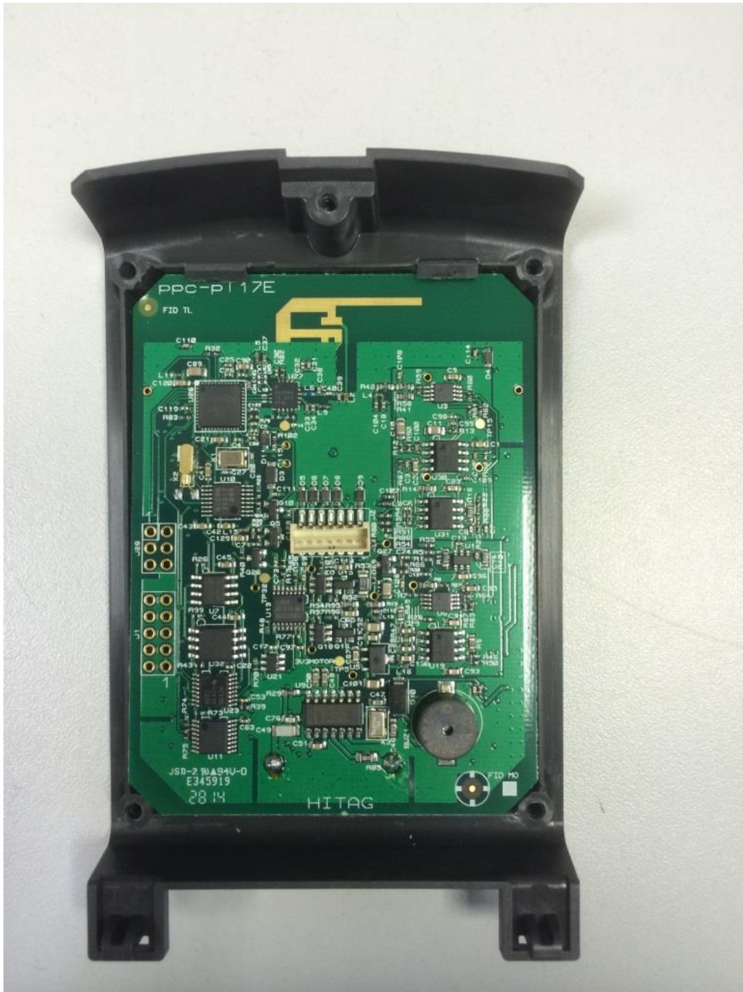
PCB in reader housing lid
