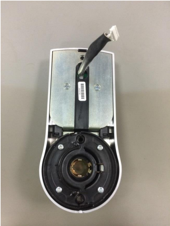
Back of insecure side enclosure – note back view of secure side enclosure is identical
