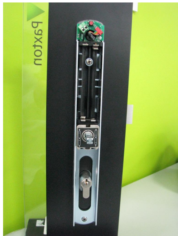
Exit unit assembly – with batteries removed
