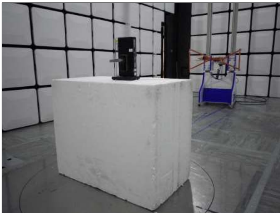
Figure 25 - Test Setup - 30 MHz to 1 GHz
