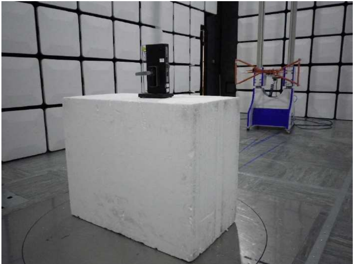
Figure 1 – Test Setup Photos 30MHz to 1GHz
