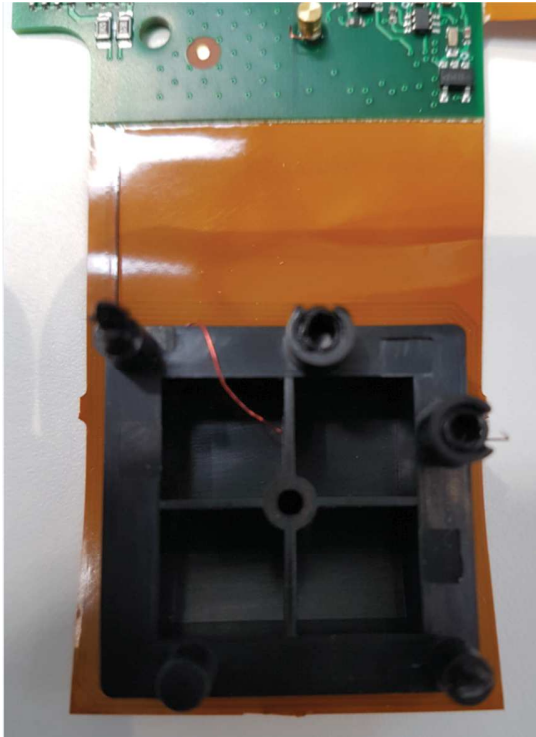
Figure 22 –Rear view of Radio Module coil housing opened out from main PCB
