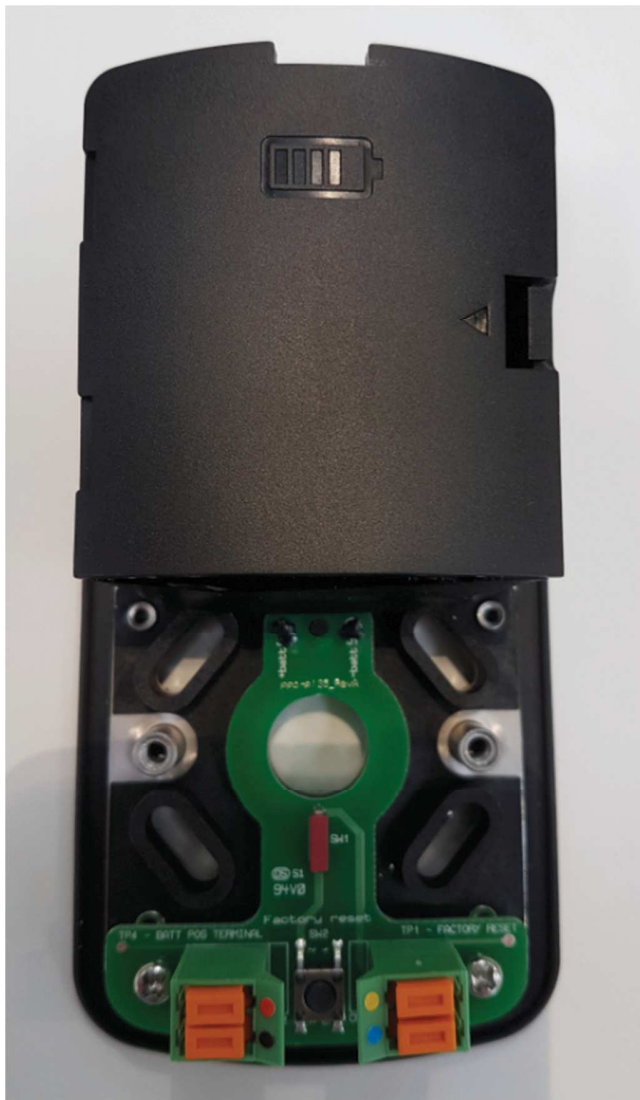
Figure 4 – Front view with Battery compartment and PCB
