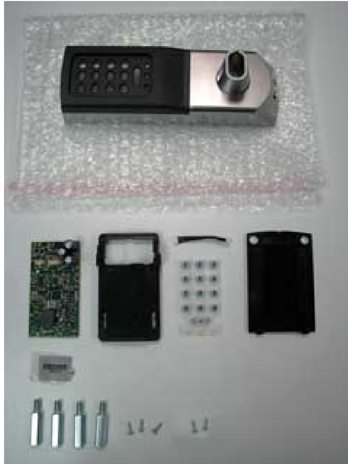
Door entry unit – main parts
