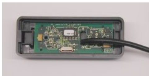
PCB & coil former in reader housing
