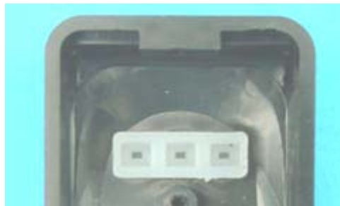
LED lens in reader housing
