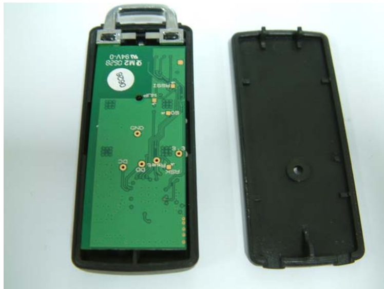
Keyfob PCB inside housing
