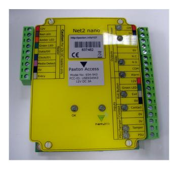
The FCC-ID and ratings labels are located on the wiring label.
