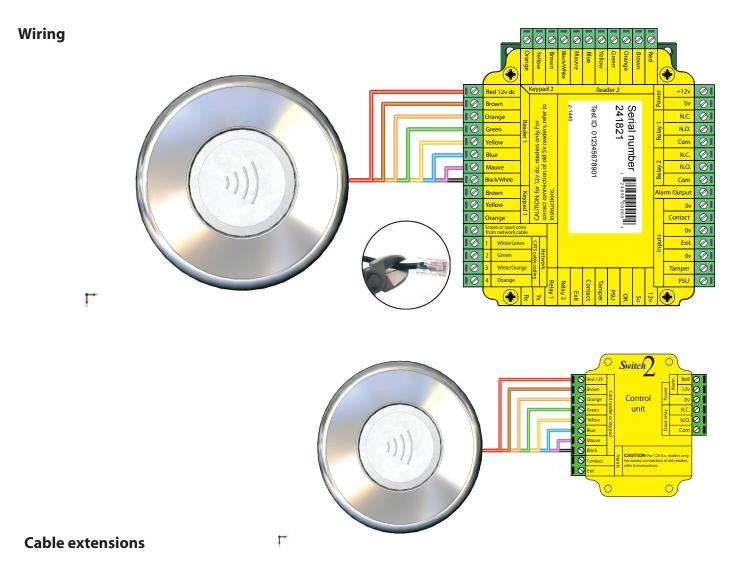
Readers can be extended using Belden CR9540 10-core overall screened cable. The maximum cable length between reader and control unit is 100 yards.
