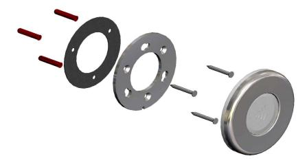
Fix the back plate to the wall with the stainlesss steel screws provided in the fitting kit. The small slot in the plate edge should be positioned at the bottom.
