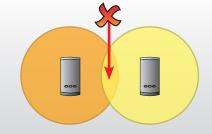
For maximum read range the Net2Air reader field should not be overlapped by the field from other interference sources at or around 125KHz. These include Loop readers, non Paxton readers, etc.
