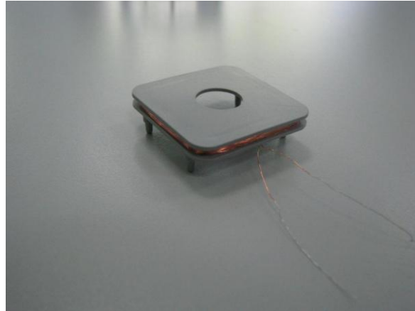
Loop antenna wound around plastic coil former
