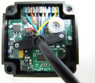
Securement of circuit board and cable clamp to reader housing with five screws.
