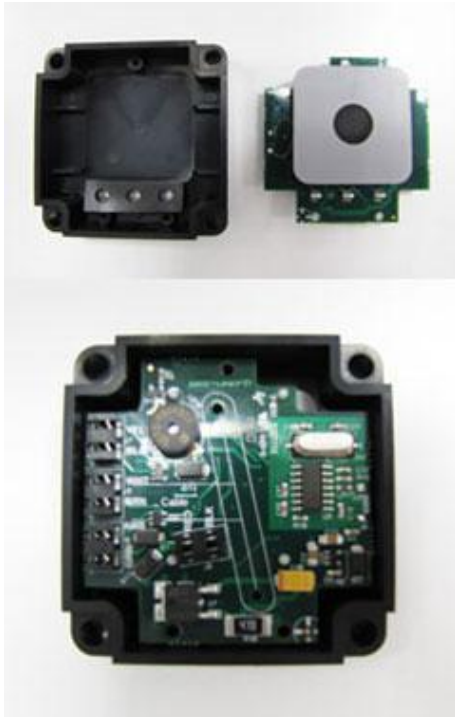
Circuit board and coil former placed inside reader housing.
