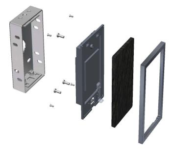
Mount the reader back box flush into the wall. Care must be taken when doing this, as there is no further adjustment possible within the box. Screws and plugs are provided for fitting the unit to the wall.
