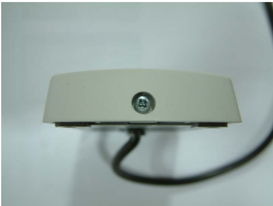
Bottom showing clip-on bezel locking screw.
