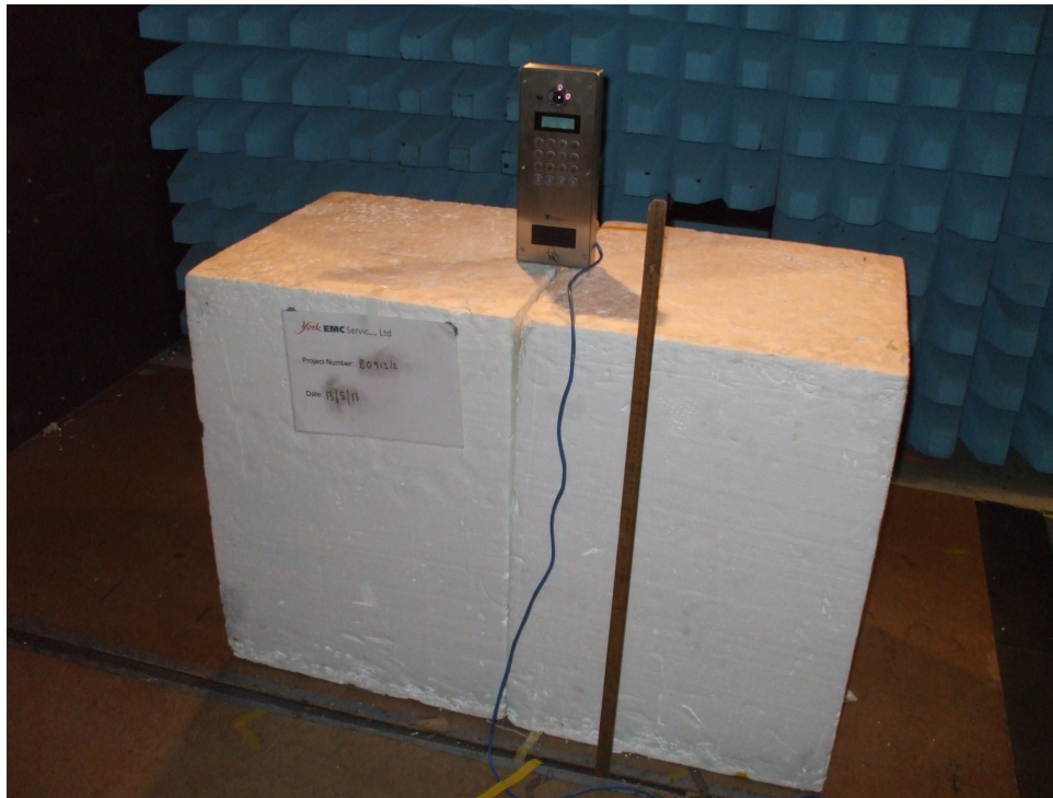
Photograph 5.3.1 Radiated emissions testing (9kHz to 30MHz), 3m, chamber
