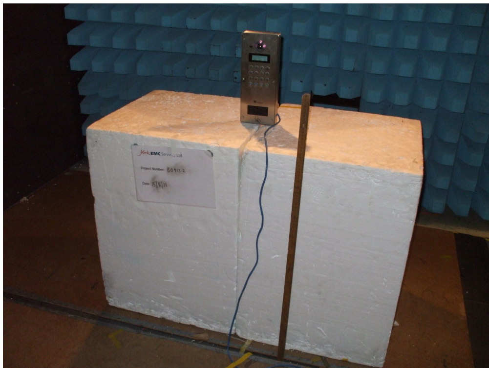
Photograph 5.3.2 Radiated emissions testing (30MHz to 1GHz), 3m, chamber
