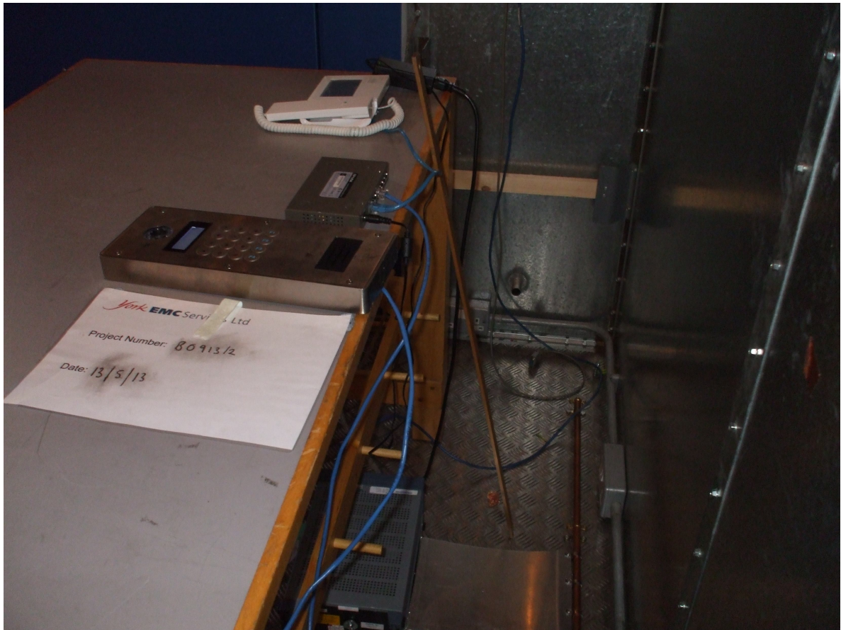
Photograph 5.3.5 Conducted emissions testing (150kHz to 30MHz)
