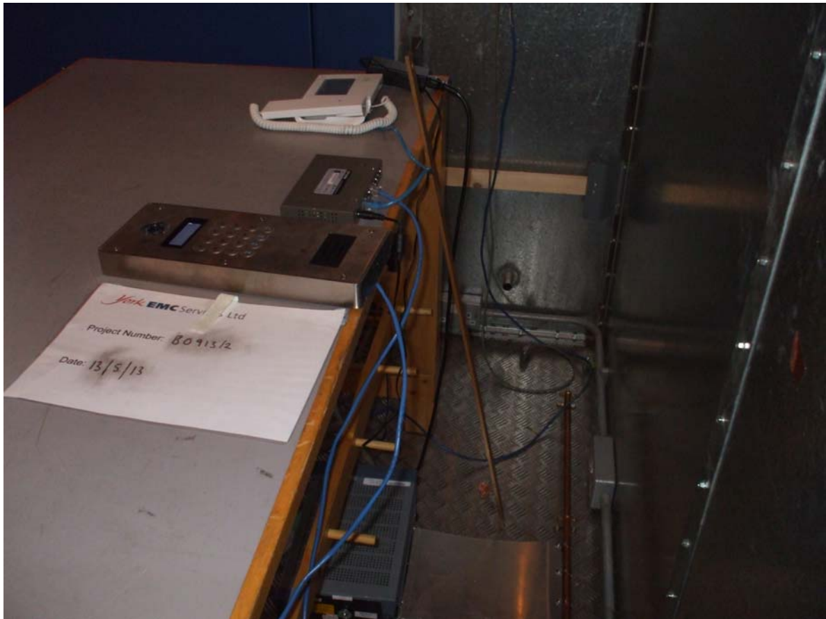
Photograph 5.3.5 Conducted emissions testing (150kHz to 30MHz)
