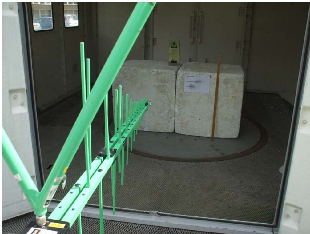
Photograph 5.3.4 Radiated emissions testing (30MHz to 1GHz), 10m, Open Area Test Site
