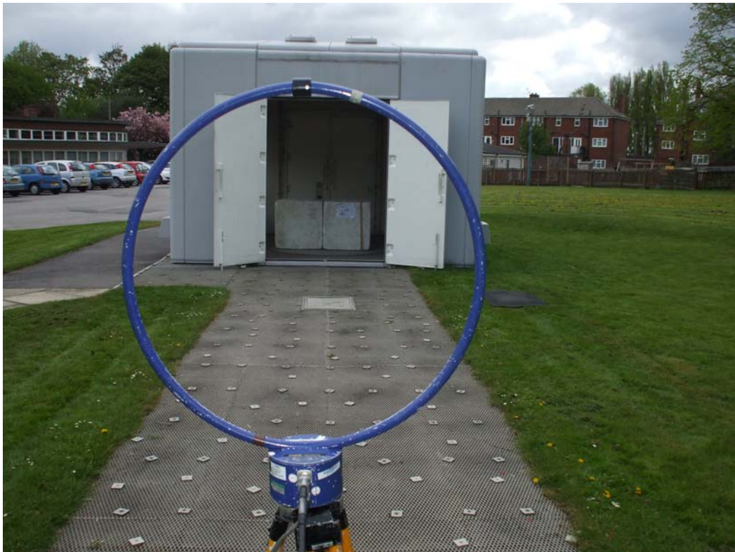
Photograph 5.3.3 Radiated emissions testing (9kHz to 30MHz), 10m, Open Area Test Site
