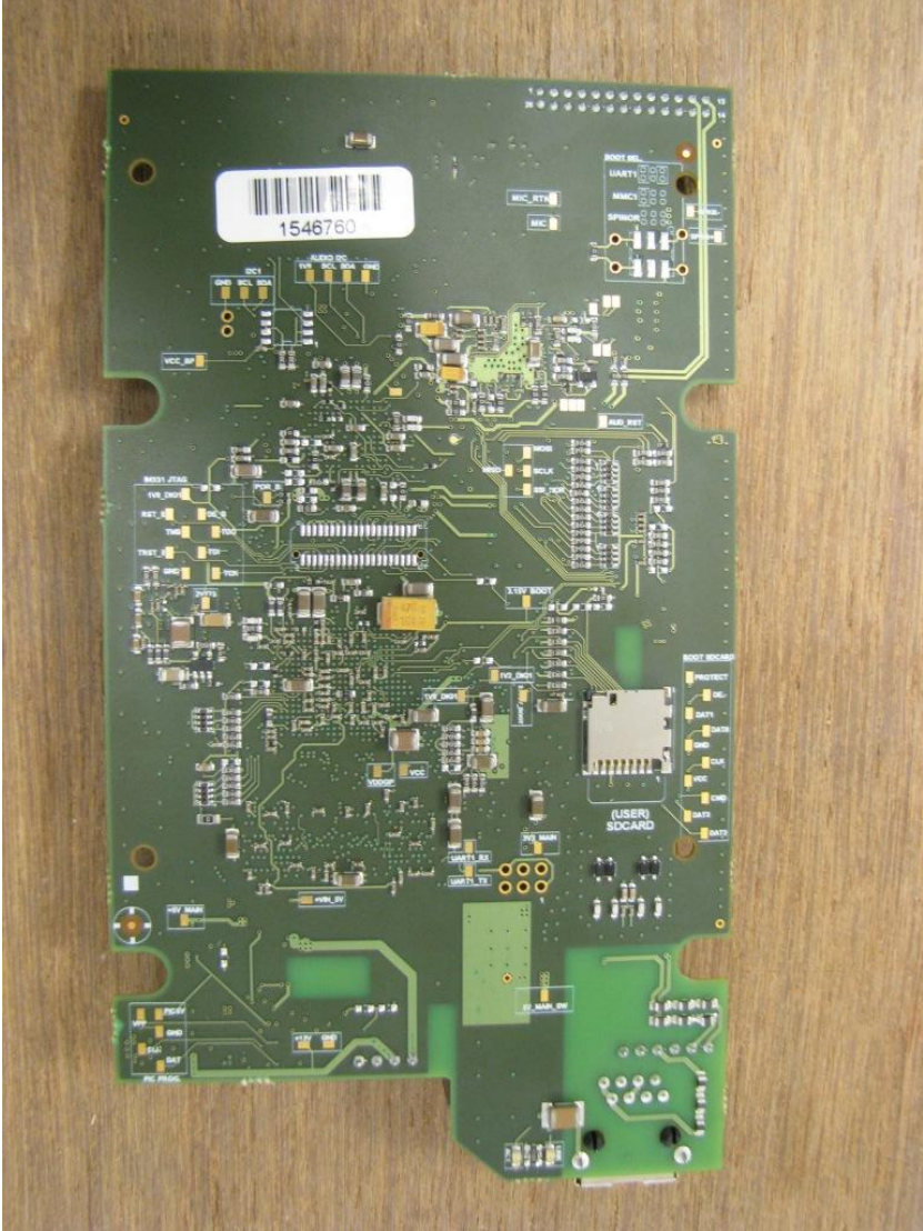
Main Panel CPU board – bottom view
