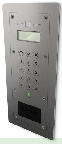
The Net2 Entry panel is a robust door entry panel incorporating both door entry and access control functions. It is powered using power over Ethernet (PoE) and communicates with the other elements of the system using IPv6, providing 'plug and play' installation. Each panel is associated with a Net2 Entry control unit which is the interface to the door hardware.
