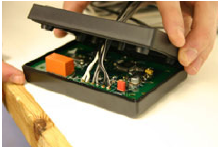
PCB & coil former in reader housing
