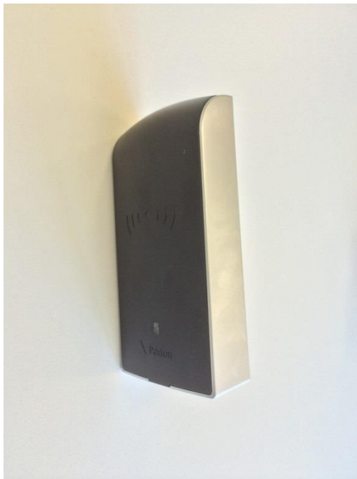
Fig 2. net10 VR reader (new variant) – outer enclosure
