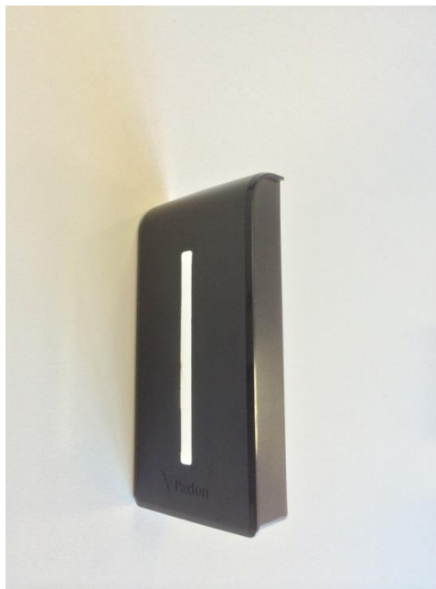
Fig 4. Clip-on cover for net10 reader as certified under USE010818 / 10217A-010818
