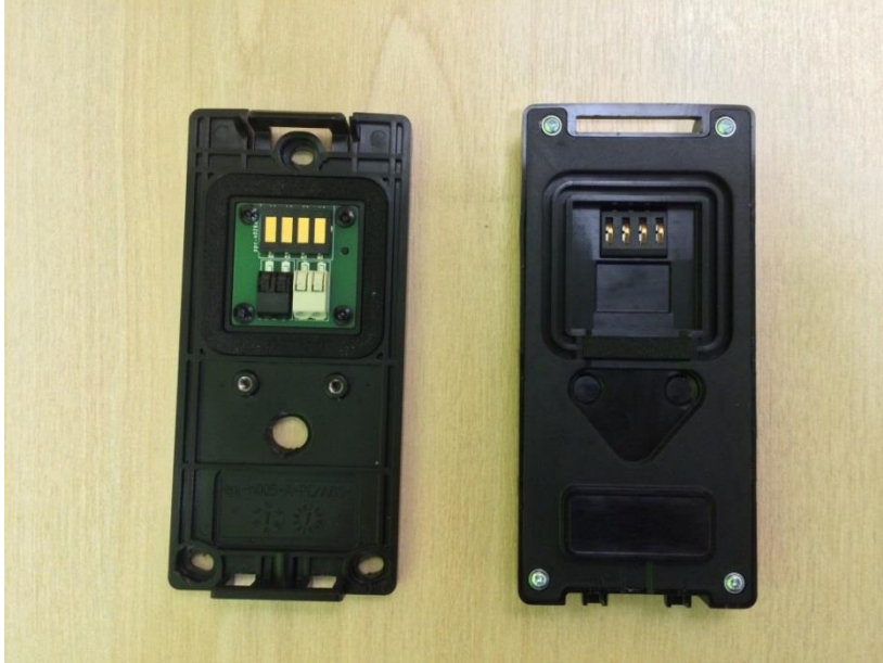
PHOTO 1 – back plate (left) and reader module (right) assemblies
