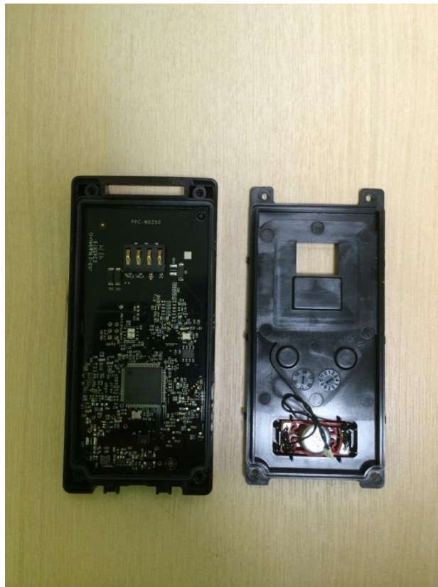
PHOTO 2 – reader module with cover removed
