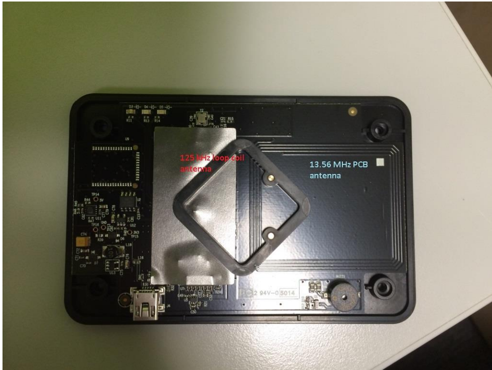
PHOTO 1 - PCB in base housing
