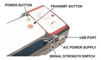
The right side of the tool has a signal strength switch that lets you select either a high-strength (70 Db) signal or a low-strength (60 Db) signal. Slide the switch up for high; slide it down for low. Next to that switch, there's an outlet for the AC power adapter. Next to the outlet, there's a port for the USB cable.
