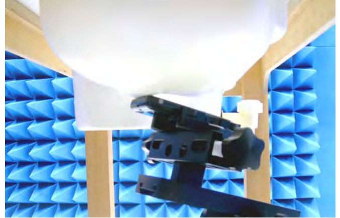
Figure 14. Right Head SAR Test Setup (Tilted)
