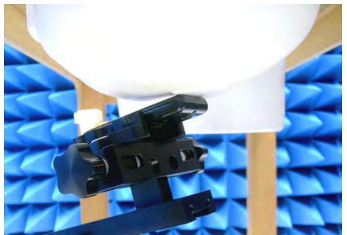
Figure 16. Left Head SAR Test Setup (Tilted)
