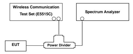
(Configuration of conducted Emission measurement)
