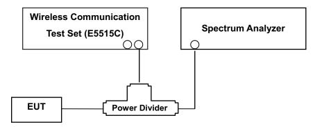
(Configuration of conducted Emission measurement) Test Procedure
