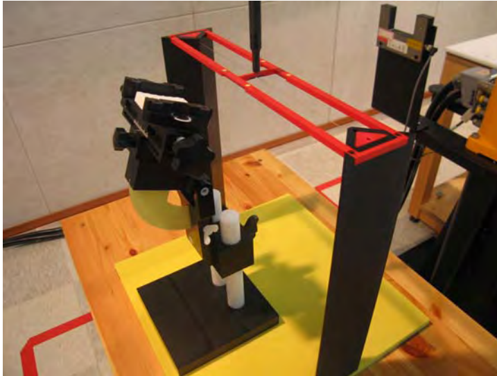
Figure 2. HAC Phantom & Device Holder
