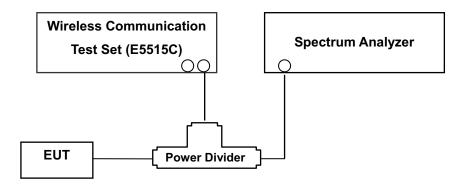
(Configuration of conducted Emission measurement) Test Procedure
