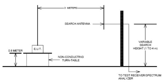
The measurement facilities used for this test have been documented in previous filings with the commission pursuant to section § 2.948. The open field test site is situated in open field with ground screen whose site attenuation characteristics meet ANSI C63.4 –2003. A mast capable of lifting the receiving antenna from a height of one to four meters is used together with a rotatable wooden platform mounted at three from the antenna mast.
