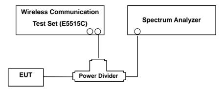
(Configuration of conducted Emission measurement) Test Procedure
