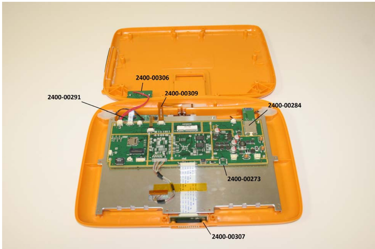
Location of 2400-00273, 2400-00284, 2400-00291, 2400-00306, 2400-00307, and 2400-00309 PCB assemblies on chassis.
