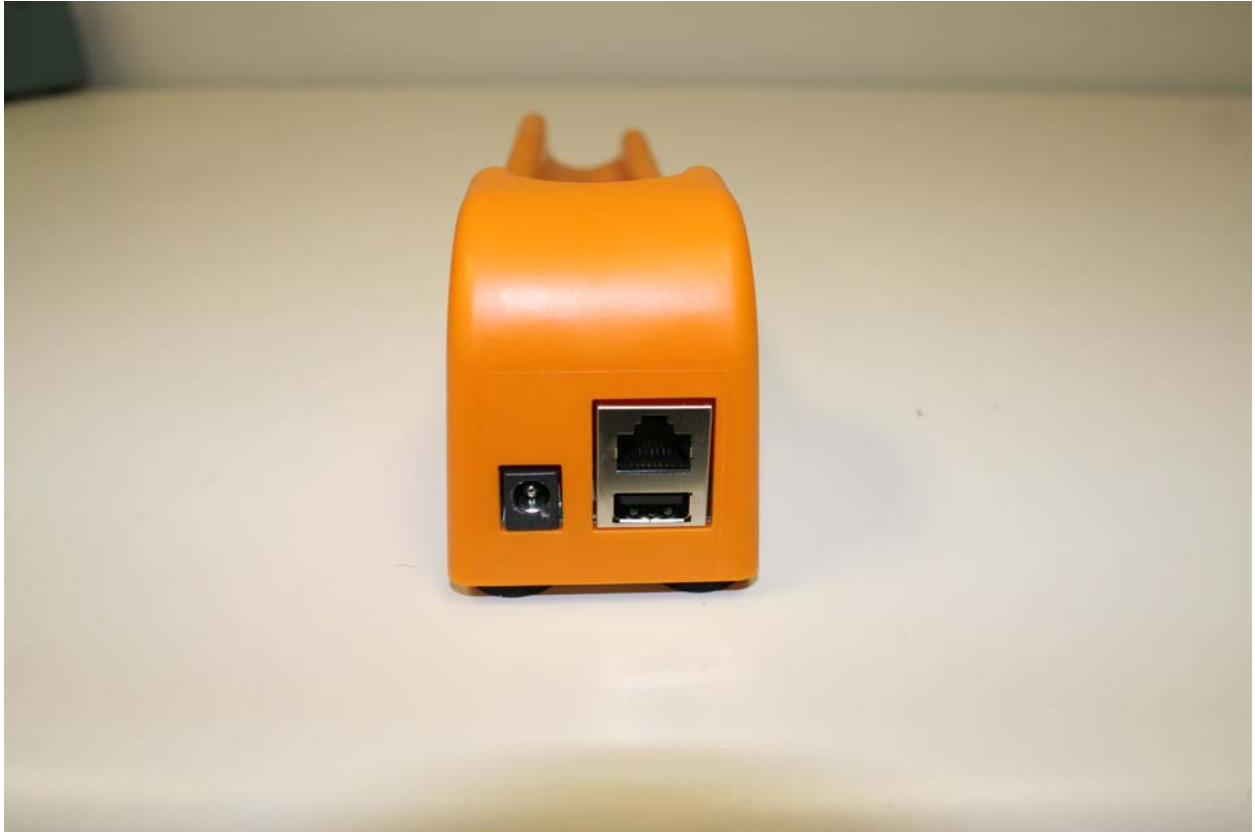
Left, showing power, Ethernet, and USB connectors
