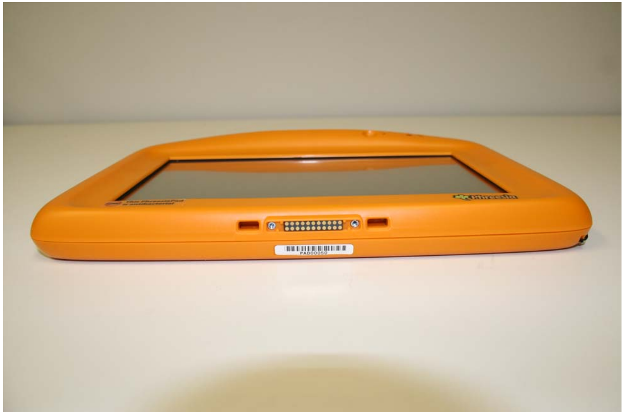
Bottom, with mating connector for Docking Cradle
