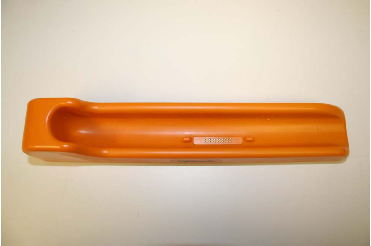
Top, showing tablet mating connector
