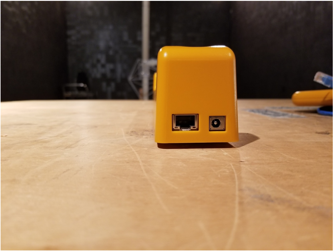
Photograph 13 - Docking cradle left side showing ethernet and power connectors
