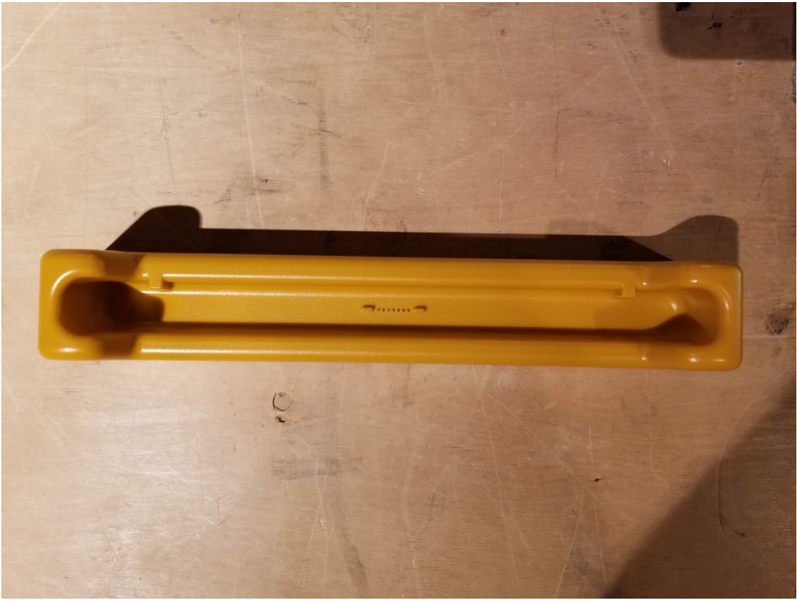
Photograph 9 - Docking cradle top showing mating connector
