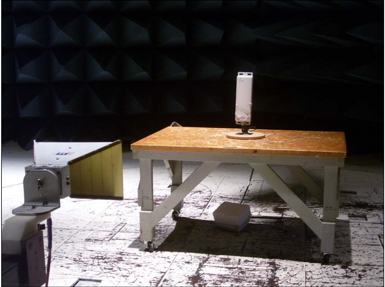
Photograph 10 Test Equipment and setup for various Radiated Measurements, HiperAccess Antenna
