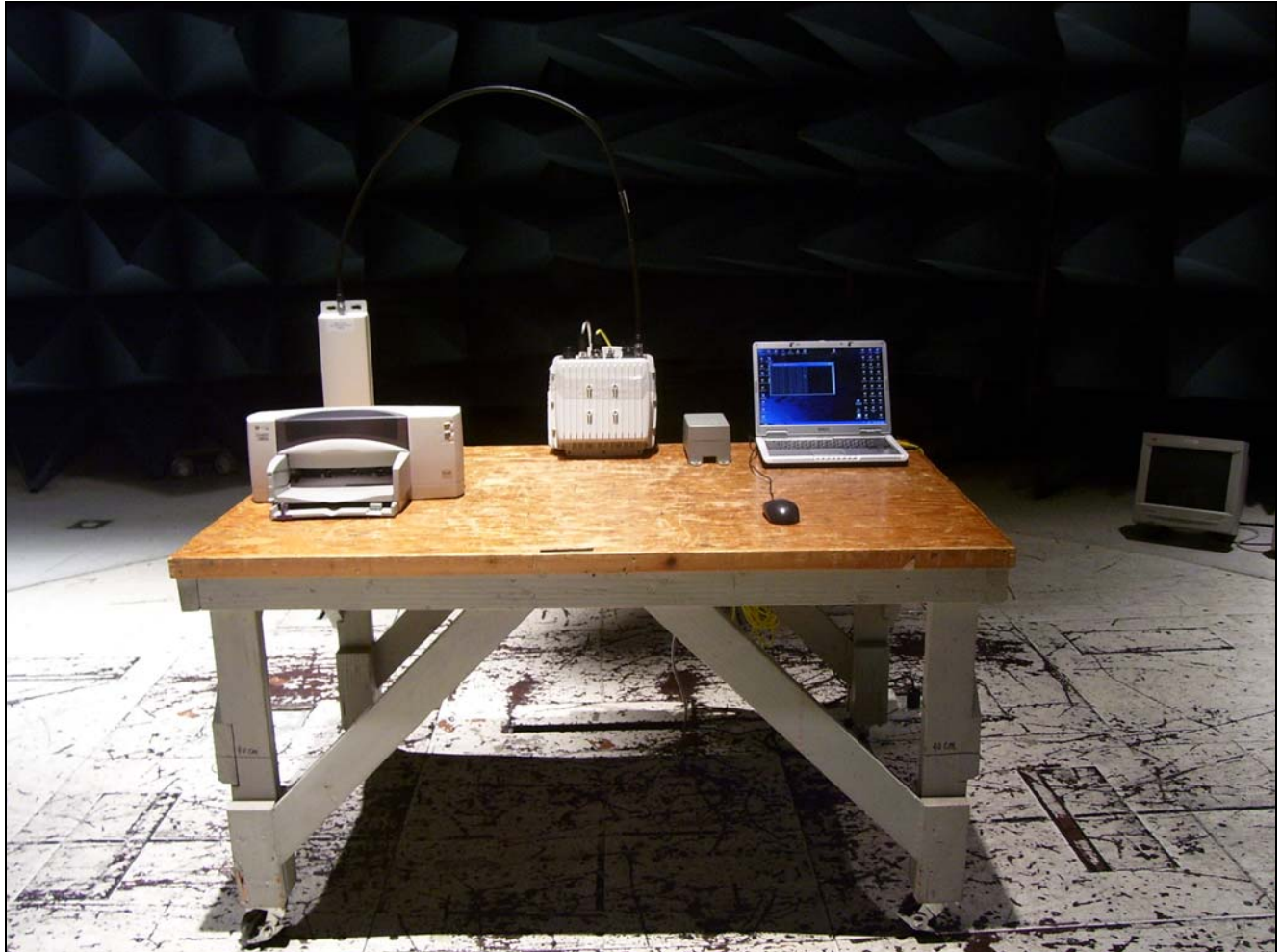
Photograph 6. Radiated Emission Test Setup 30 MHz - 1 GHz for ASN-800FCC-N
