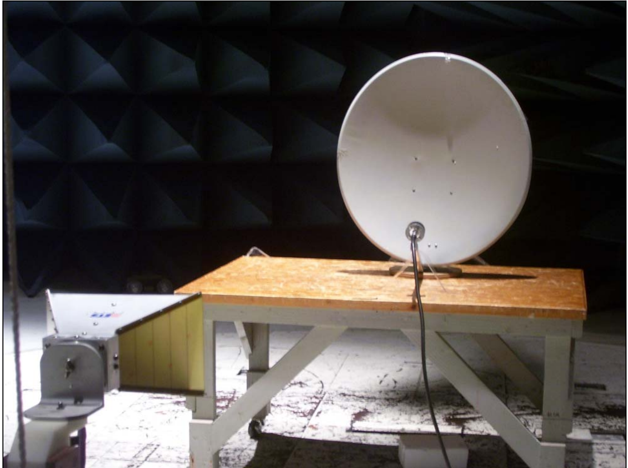
Photograph 15. Test Equipment and setup for various Radiated Measurements, 5158PP8 Antenna
