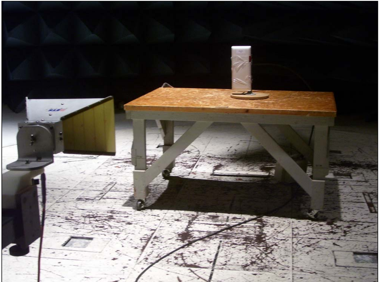
Photograph 13. Test Equipment and setup for various Radiated Measurements, MT-484033-NV Antenna
