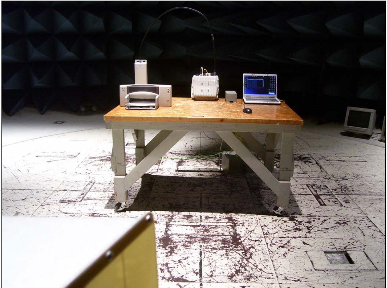
Photograph 8. Radiated Emission Limits Test Setup 1 - 5GHz for ASN-800FCC-N
