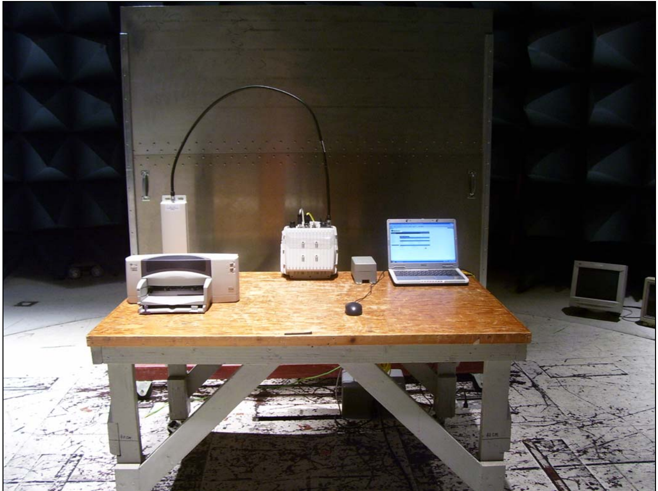
Photograph 4. Conducted Emissions Test Setup for ASN-800FCC-N
