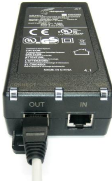
Figure 55. Installation of the (power + data) Ethernet cable to the PSU-4.
