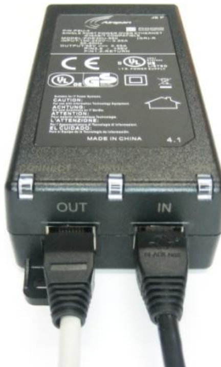
Figure 57. Installation of the Ethernet cable to the "IN" port of the PSU-4.
