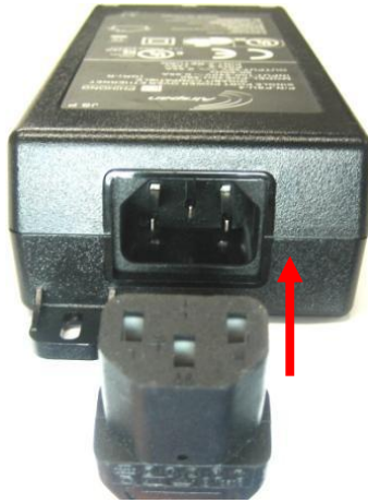
Figure 42. The installation of the AC power cable to the PSU-4.
