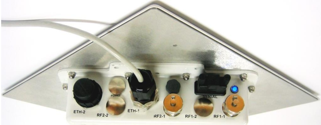
Figure 56. Installation of the (power + data) Ethernet cable to the ETH-1 port of the FlexNET unit (ASN-900P).
