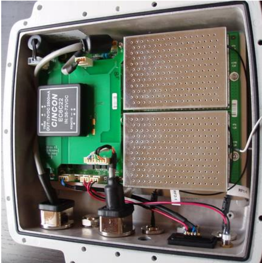
Inside of ASN-900 with shielding cans fitted
