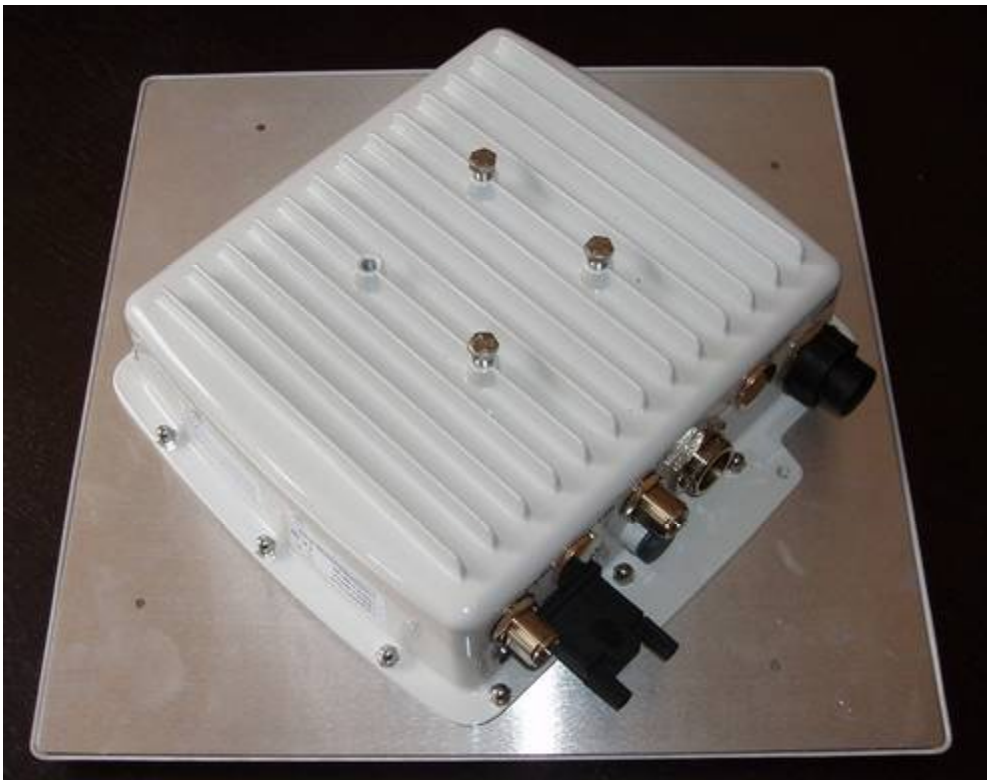
External photo showing connector face and label face of casting
