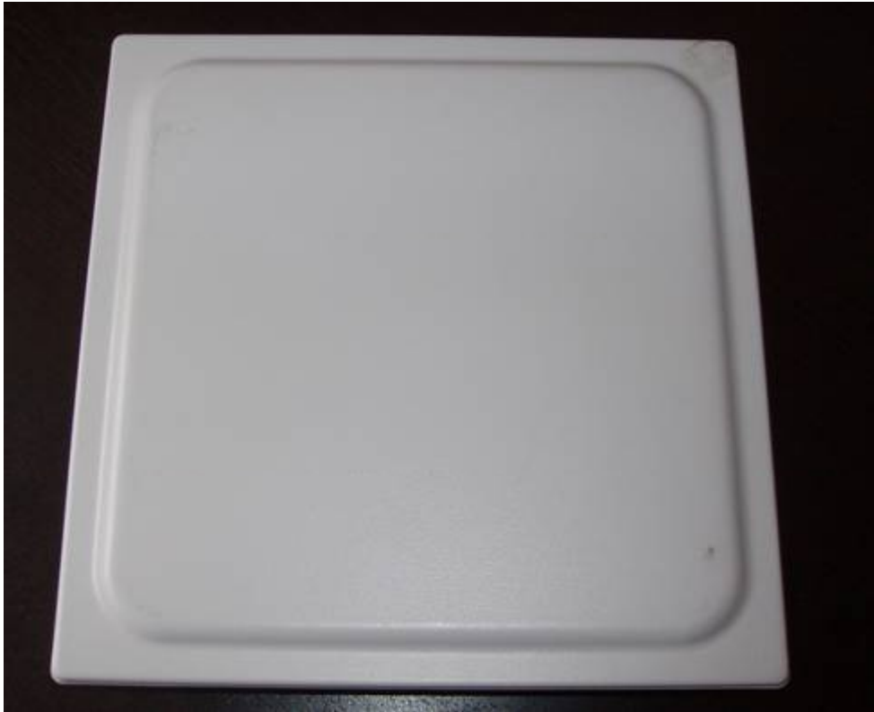
External photo showing radome on 23dBi integral antenna
