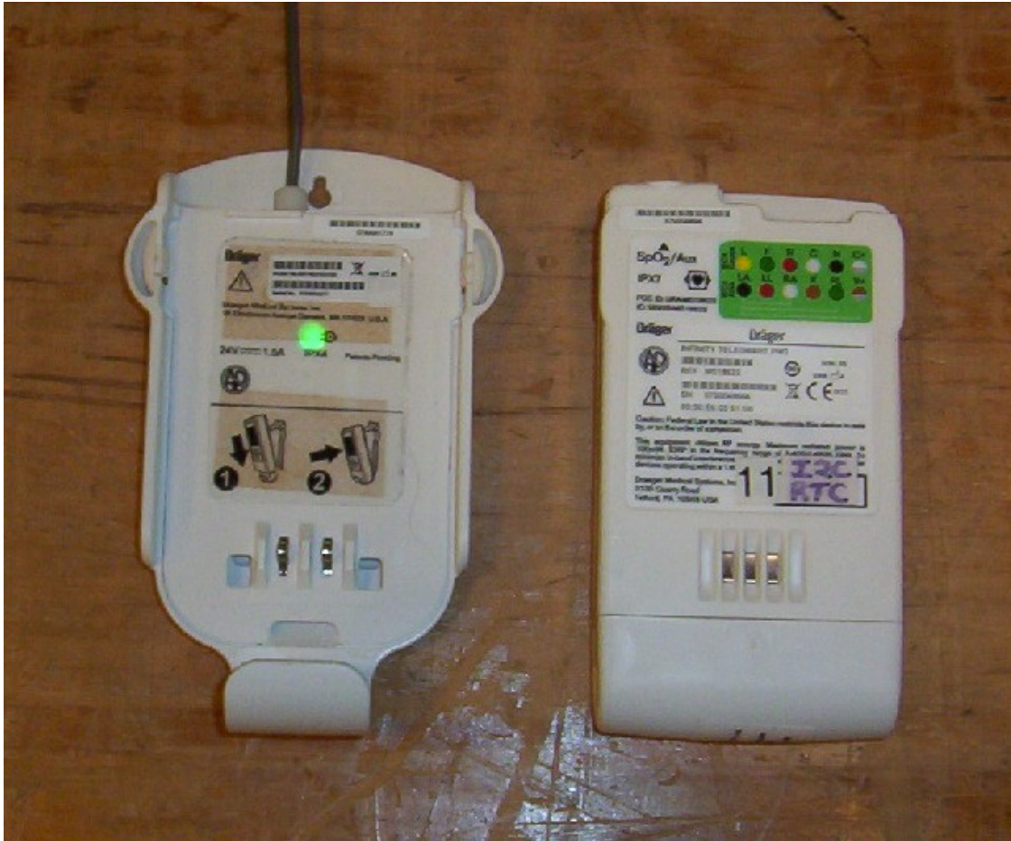
Figure 2 – Docking station on left and back of EUT on Right
