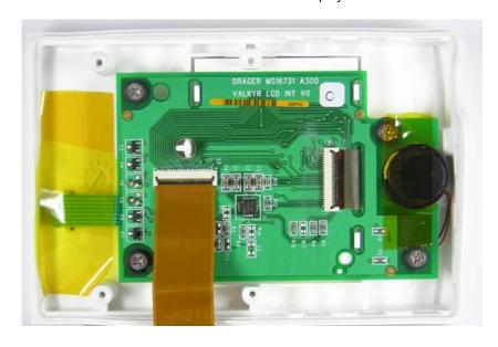
Internal Photo Top view of PCB from Display
