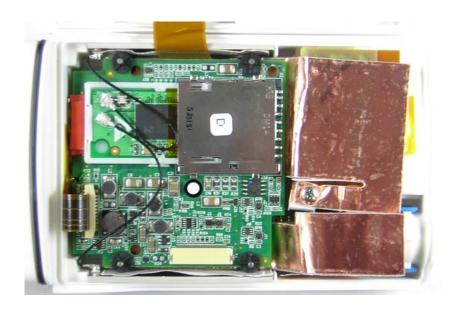
Internal Photo Rear view of PCB with RF-module
