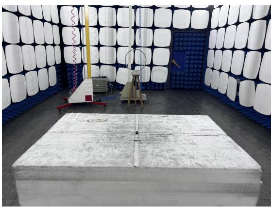
3. Radiated emission (9KHz-30MHz)
